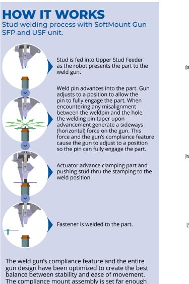
from the weld plane that it does not introduce variation to the welding process itself.
